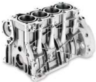
High pressure die cast deep skirt block of the Daimler A class in-line 4-cylinder engine with cast-in grey iron liners Source: KS ATAG
