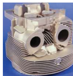
Air-cooled cylinder head cast from Al-12Ce
