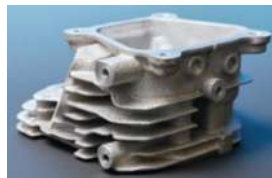
Air-cooled cylinder head cast from Al-12Ce-0.4Mg
