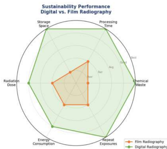
Figure 2: Sustainability Performance Comparison — Digital vs. Film Radiography across six key dimensions.
