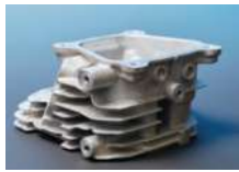
(iii) Air-cooled cylinder head cast in Al-12Ce-0.4Mg
